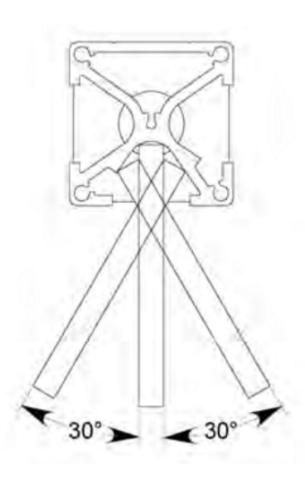
The multi-function insert component provides the ultimate versatility for custom projects allowing you to adjust your glass height and angles (up to a 60 degree variance) for a nearly limitless range of options for your outdoor designs.
