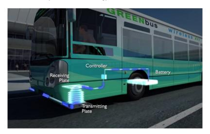
ORNL researchers will explore innovations to increase power transfer level to 200 kW and eventually 350 kW, while refining dynamic wireless charging technology. A dynamic system enables the automatic charging of electric vehicles using wireless charging pads installed under roadways. Higher power charging systems are needed to minimise the cost and complexity of dynamic charging. "The goal is dynamic charging at highway speeds," Galigekere said.
