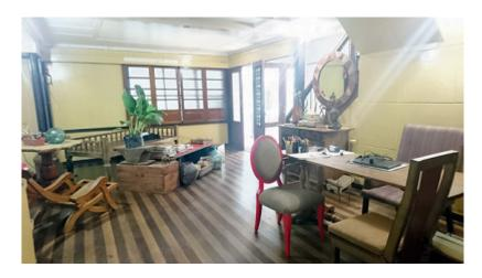
Engineered wood planks are not real wood planks. They consist of a hardwood core with a layer of hardwood veneer fastened using adhesives at the top surface. One advantage of this material is that it is sturdy and humidity-resistant. Another is that this variety is a less expensive alternative to genuine hardwood floors.
