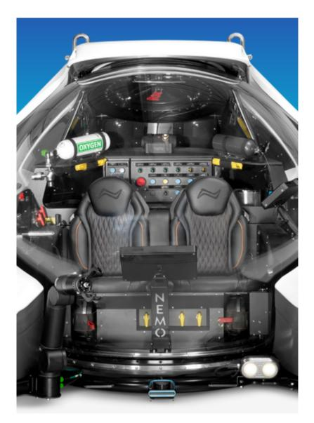
It's an air conditioned, transparent acrylic bubble with a handheld controller for maneuvering at depths as far down as 100 meters or about 328 feet.
