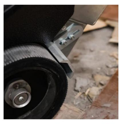
This movement can be controlled with the innovation of a dial allowing for oscillation adjustments. It's switched off for easily removed materials and it's switched on for difficult to remove materials. Maneuverability is a feature in a walk-behind surface scraper that improves speed and efficiency.
