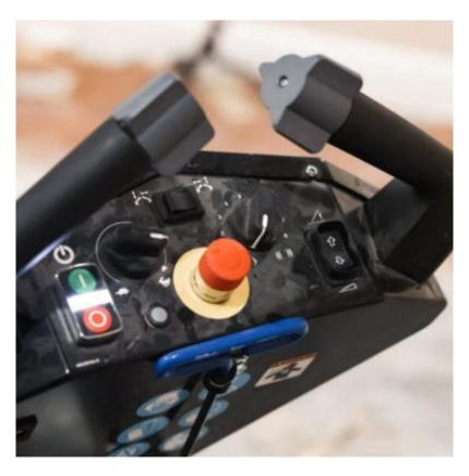
So. How does it work? The toggles on the handle direct The Rogue left, right, forward or reverse. Unlike most machines, it has a button, which conveniently controls the blade's pitch and angle; where pitch and angle adjustment is not significantly limited by a few different attachment options. The machine's vibration is used to improve machine efficiency. Tooling on machinery oscillates or moves or swings back at a regular speed, which is productive in the removal of surface material.
