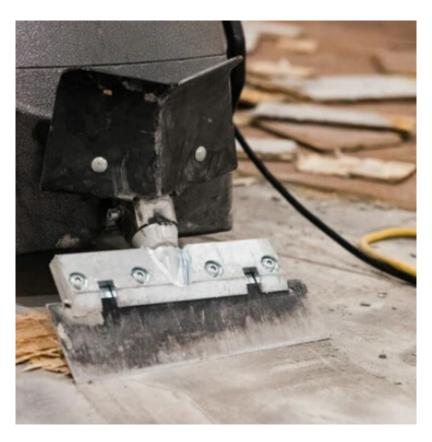
The Rogue is an electric machine that delivers increased maneuverability and speed for the user. Instead of 30 feet per minute (some walk-behind scrapers), it scrapes up to 150 feet per minute and is easier to use with simple controls, which require less operator attention than most models.
