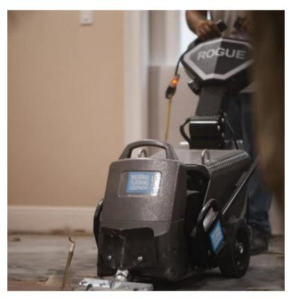
What makes this machine unique? It provides the power and the productivity of a ride-on scraper within the compact size of a walk-behind. The challenge with maneuvering most ride-on scrapers is that they require the use of hydraulics. Operating The Rogue does not require using hydraulics.
