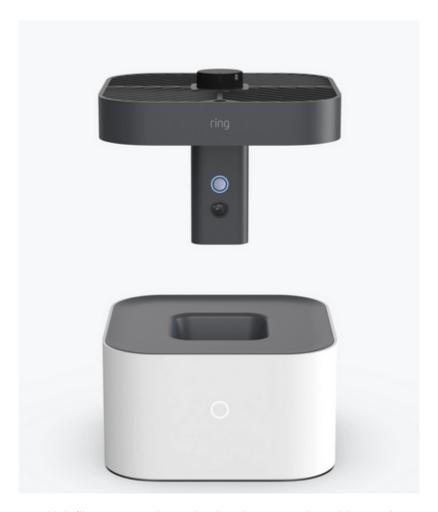
This aerial indoor camera, which flies on a predetermined path when activated by an alarm sensor, was unveiled in September 2020. It uses light detection and ranging (LIDAR) laser sensors to create a flight path around you home; the scheduled launch date of this product is currently unknown.
