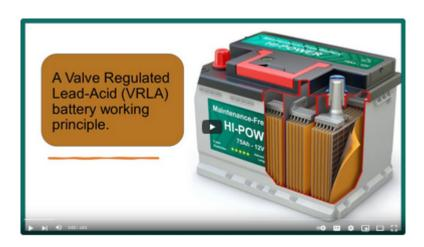
A valve regulated lead—acid (VRLA) battery or sealed lead—acid (SLA) battery, is characterized by a limited amount of electrolyte ("starved" electrolyte) absorbed in a plate separator or formed into a gel. The negative and positive plates are proportioned so that oxygen recombination is facilitated within the cell. A relief valve retains the contents independent of the position of the cells.
